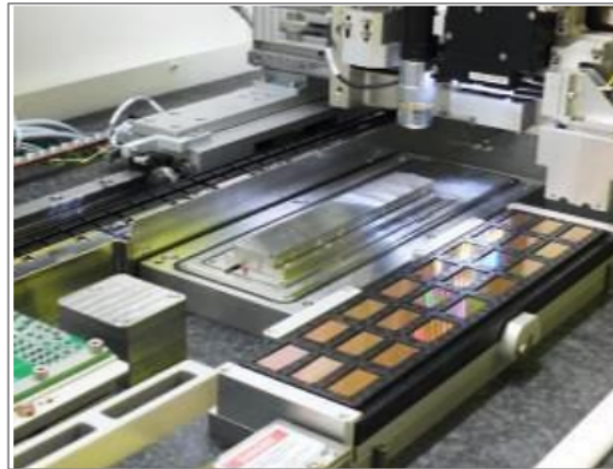
Fig.2 View of central area of the machine, HIC assembly table and chips tray
